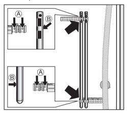
Secure the transit bars to the back of the washing machine. Make sure that holes (B) are fitted over retainers (A). The washing machine must not be moved without the transit bars in place.
